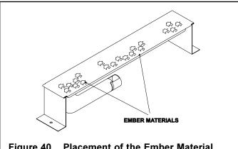
Figure 40. Placement of the Ember Material
